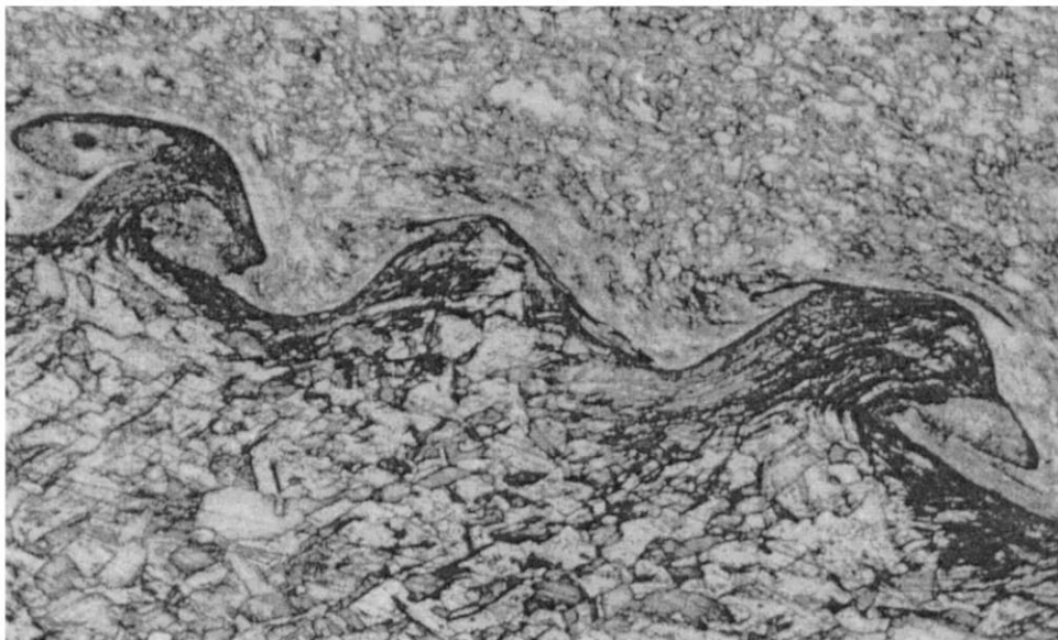
Fig. 10. Appearance of interface in model experiment of Fig. 9: (a) central region which underwent normal impact; (b) lateral region.
